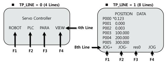
As shown in the figure, move the 4th or 8th line in Teach pendant to the corresponding menu using 'Mode Selection Button' in TP.
